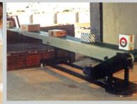
Telescopic Belt Conveyor being multistage, can be ideally used in loading bays, shipping areas where space is a constraint. It reaches to the end of the vehicle providing smooth uninterrupted flow from the beginning to the end of the truck / container.
